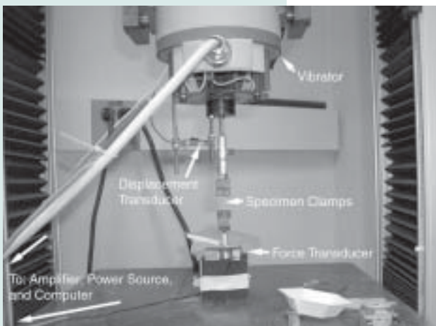
Instrumentation used to test the mechanical properties of egg capsule material. Photo: Scripps Institution of Oceanography
